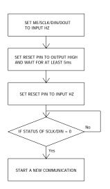
After set the host MCU's reset interface pin is set to input HZ, the host MCU can check the status of SCLK/DIN before starting a new command.
